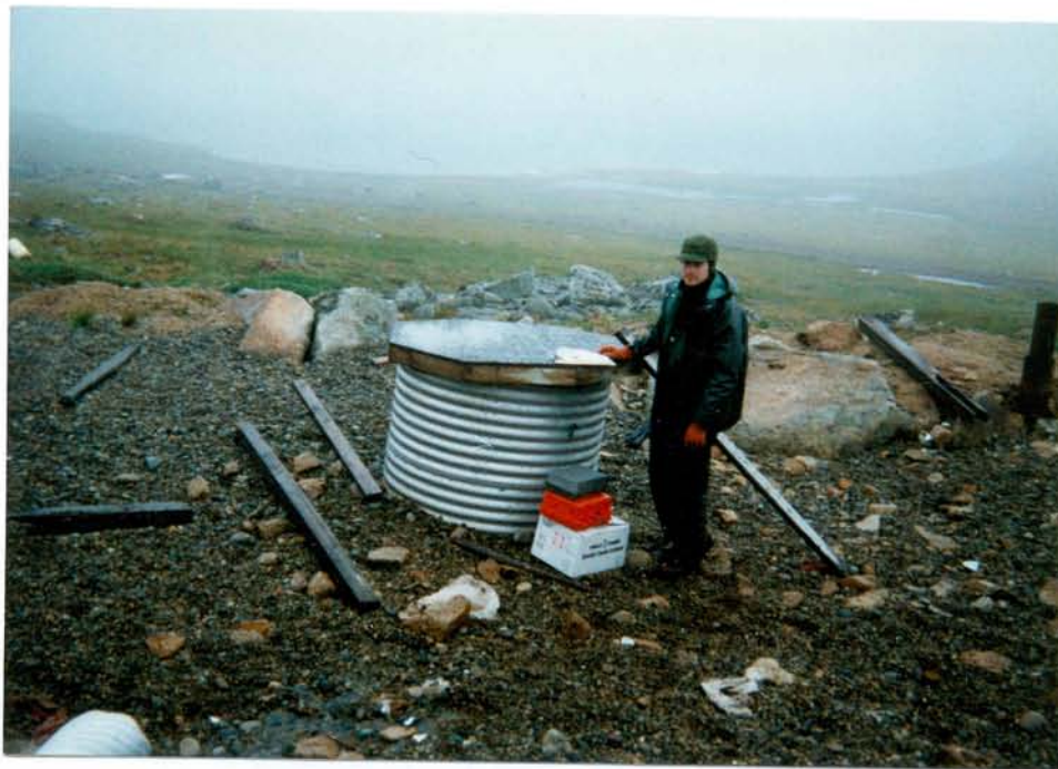
Water sampling of infiltration gallery for PCBs and BTEX. Sample #96GAMPMPHS003
