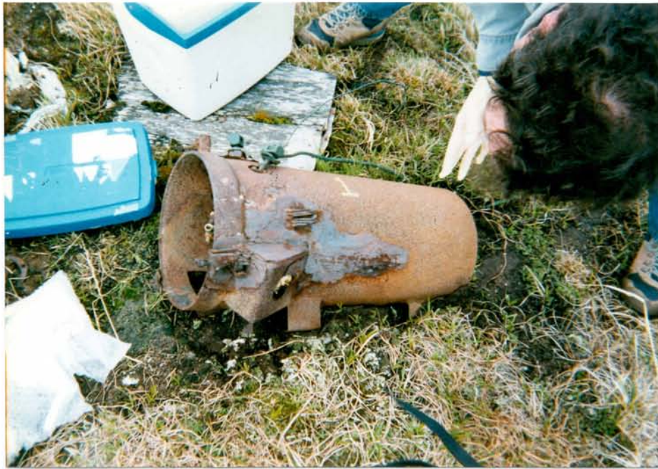
Wipe Sampling at Transformer 1 at Site 4/Area 4D. Sample #96GAM001WI
