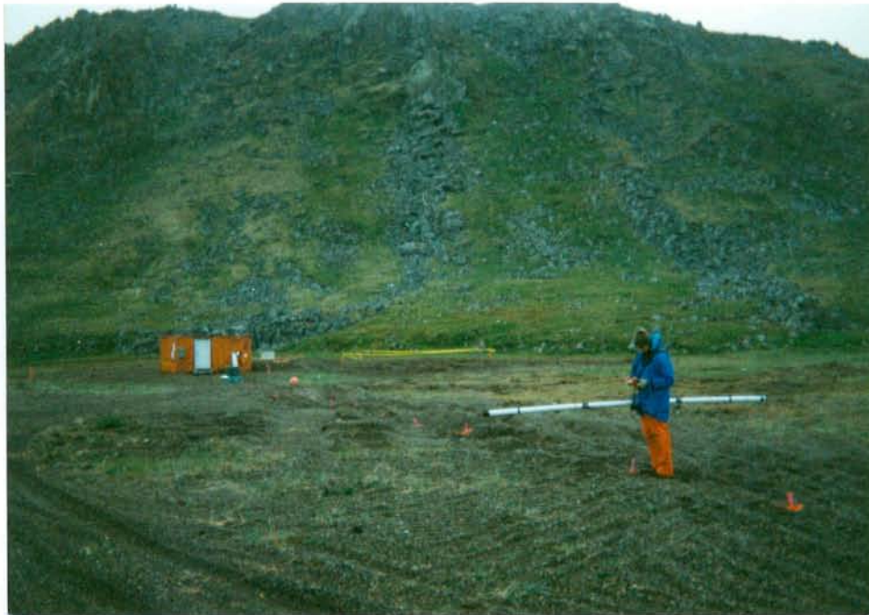
Ian Bishop (Golder Assoc.) performing EM-31 over Site 5 Geophysical Grid.
