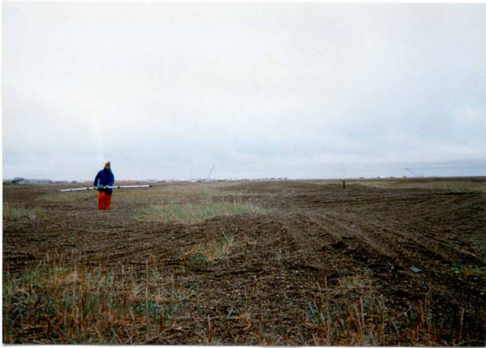
Ian Bishop (Golder Assoc.), performing EM-31 survey site of reported ammunition location.
