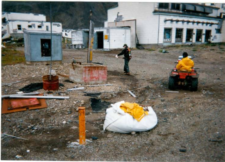
Site 27 looking South. Note: MW 27-1 and staining
