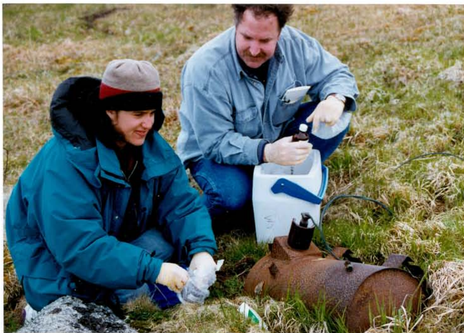
Victor Harris and Elise Tuzman (Montgomery Watson) wipe sampling of Transformers at Site 4/Area 4D
