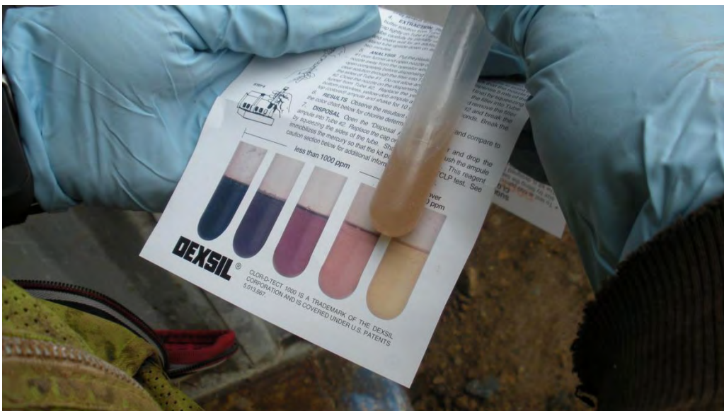
Running Chlor-D-Tect 1000 chlorine halogen test kits on reclaimed oil.
