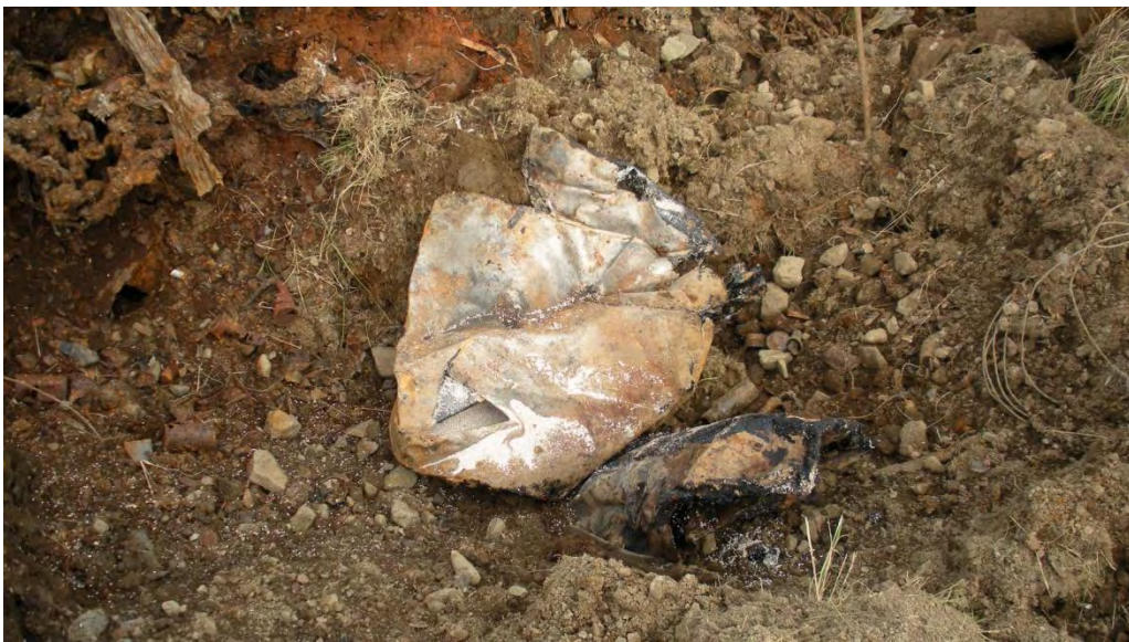
Crushed drum with sticky sludge/oil, cleaned of gross outer and reachable inner sludge, and lined inside and out with kitty litter.
