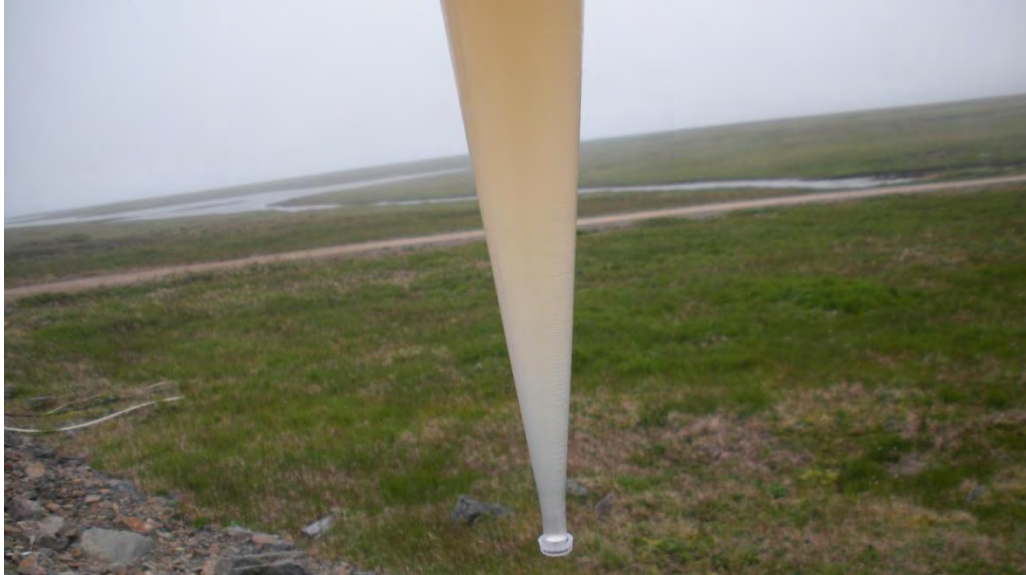
Water from final containment area shown in Imhoff cone, no settleable solids were observed.
