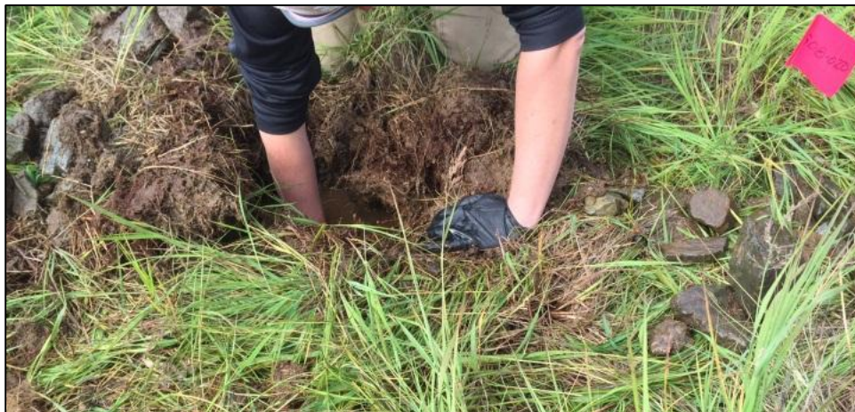
Photograph 5-6: Collecting sample SS-020 at Site 8, a saturated surface soil of coarse gravel and sand below cobbles on 18 August 2016; this sample was collected from the LDU near the MDU boundary. View facing down.
