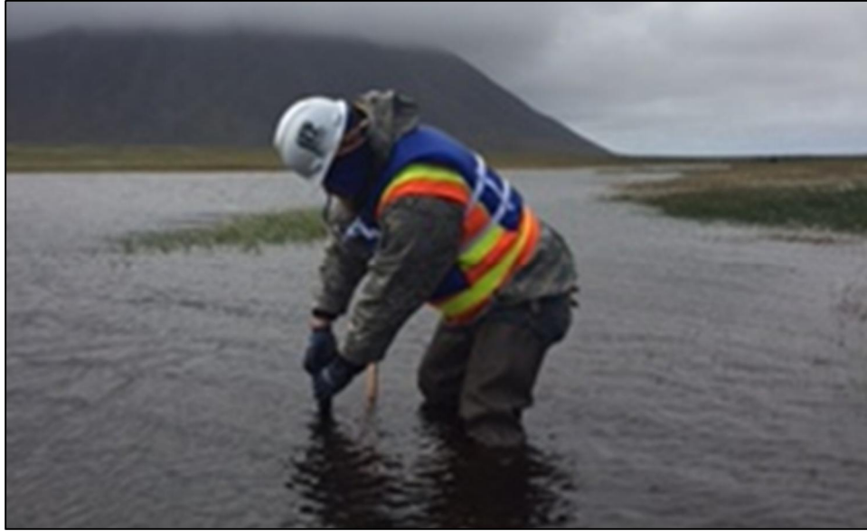
Photograph 5-7: Collecting sediment from cross-section S29-SD-010 with a hand auger on 15 August 2016. View facing south, flow to the northeast.
