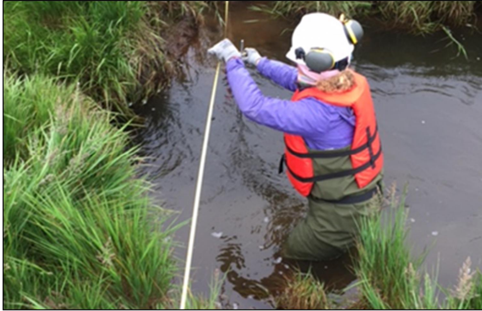
Photograph 5-11: Collecting flow measurements at the midpoint of the Suqi River at Cross-Section S29-002 on 16 August 2016. View facing down, flow to the west (right).
