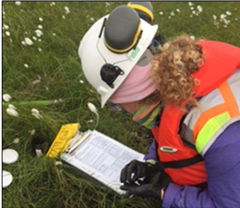
Photograph 5-9: Classifying sediment using the USCS chart at Cross-Section S29-010 on 15 August 2016. View facing down.
