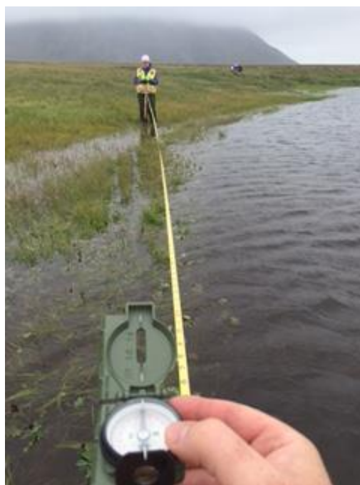
Photo No. 14 – 15 August 2016; 1522 hours. Method used to locate actual proposed sample location for S29-006 in Suqi River estuary. Facing south, flow to the northeast.
