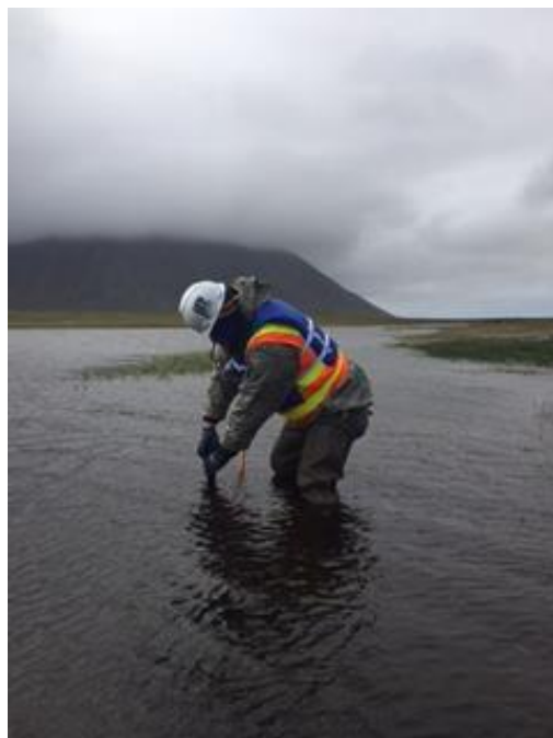
Photo No. 11 – 15 August 2016; 1305 hours. Collecting sediment from S29-010 in Suqi River estuary with hand auger. Facing south, flow to the northeast.
