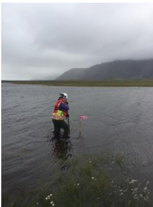
Photo No. 10 – 15 August 2016; 1258 hours. Collecting sediment from S29-010 in Suqi River estuary with hand auger. Facing southeast, flow to the northeast.
