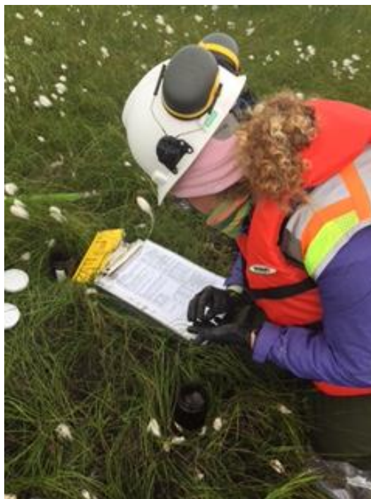
Photo No. 12 – 15 August 2016; 1316 hours. Classifying sediment from Suqi River estuary using a USCS chart at S29-010. Facing down.
