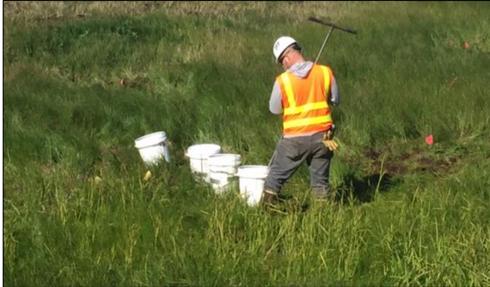
Photograph 5-4: Decontaminating sample collection equipment during sediment and soil sampling at Site 8 on 17 August 2016. View facing west.
