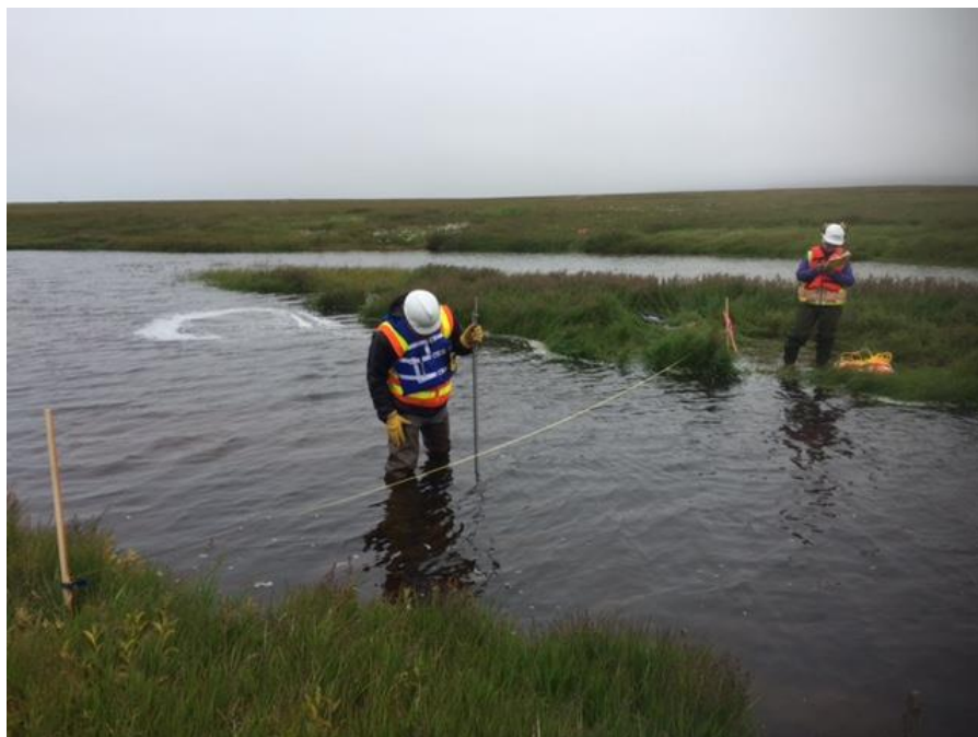
Photo No. 21 – 16 August 2016; 1524 hours. Collecting depth measurements along the tag line at Suqi River cross section S29-004; while the source of the downstream foam was not investigated, it is likely the result of natural decomposition. Facing northeast, flow to the northeast.
