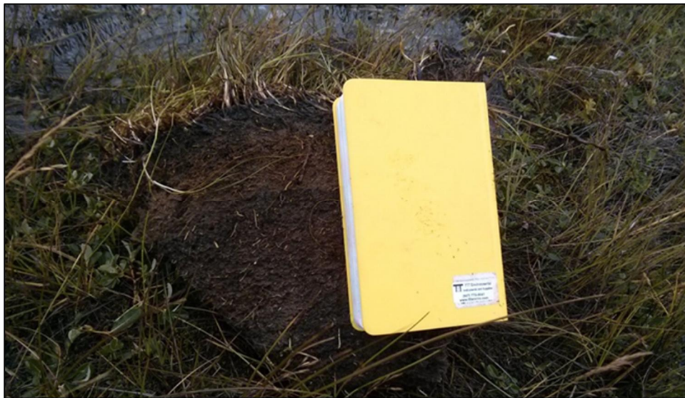
Photograph 5-8: Organic layer encountered and removed prior to sampling sediment at S29-SD-009 on 15 August 2016. View facing down.
