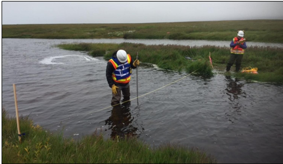
Photograph 5-10: Collecting depth measurements along the tag line at Cross-Section S29-004 on 16 August 2016; while the source of the downstream foam was not investigated, it is likely the result of natural decomposition. View facing northeast, flow to the northeast.
