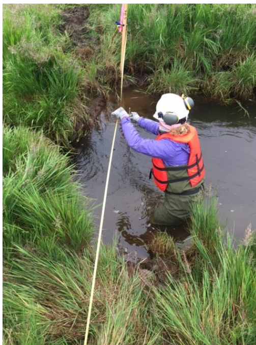
Photo No. 23 – 16 August 2016; 1641 hours. Collecting the depth measurement at the midpoint of the Suqi River at cross section S29-002. Facing down, flow to the west (right).
