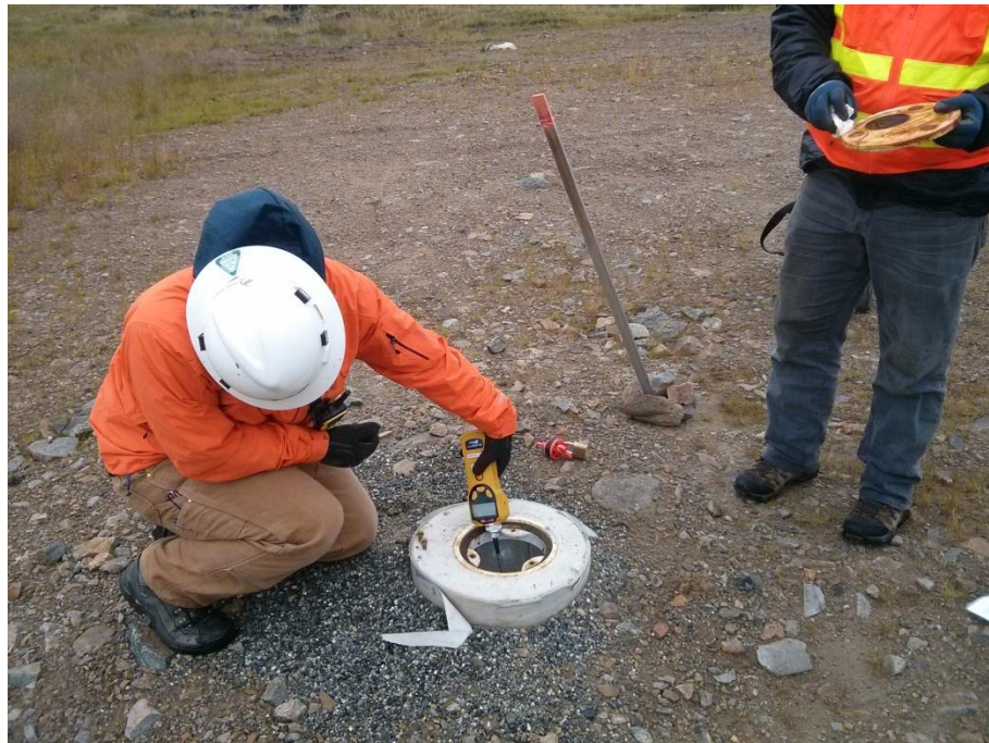
Photo No. 6 – 10 August 2016; 1216 hours. Collecting in well air measurement using a PID at well 14MW04. View facing south.
