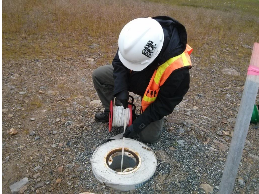
Photo No. 7 – 10 August 2016; 1217 hours. Typical collection of groundwater depth at a monitoring well; well 14MW04. View facing down.
