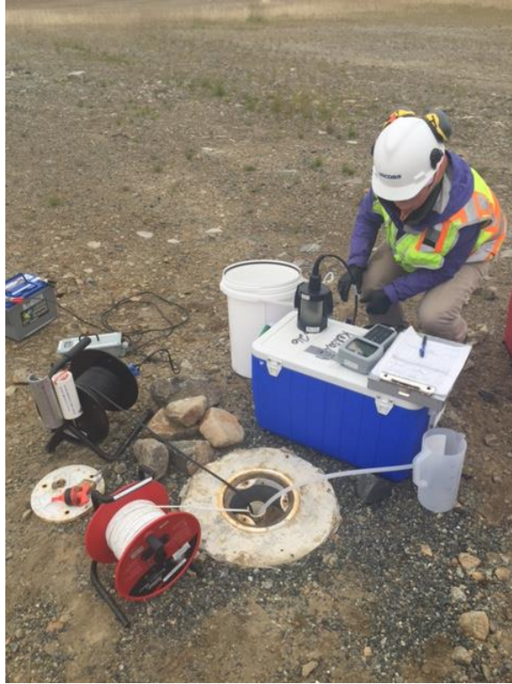
Photo 5-5: Purging groundwater at Monitoring Well 14MW01. View facing southeast.
