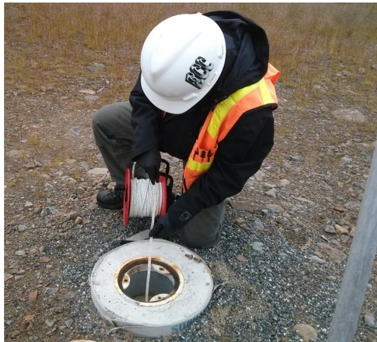
Photo 5-4: Typical collection of groundwater depth at a monitoring well; well 14MW04. View facing down.
