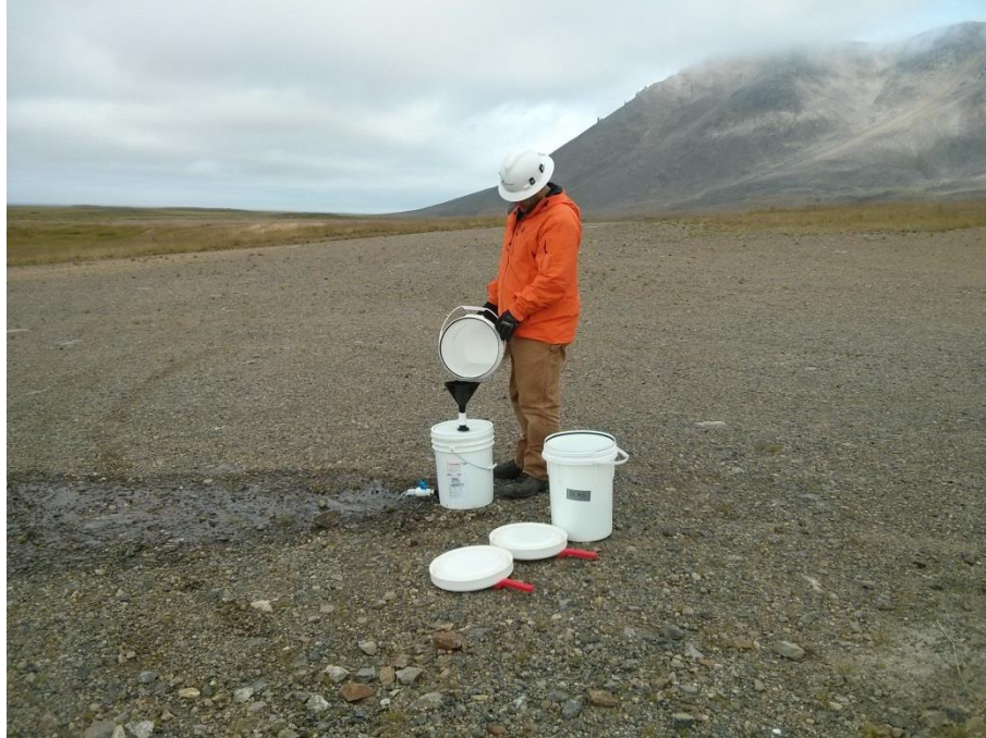
Photo No. 11 – 13 August 2016; 1918 hours. Using GAC filter on-site. View facing east.
