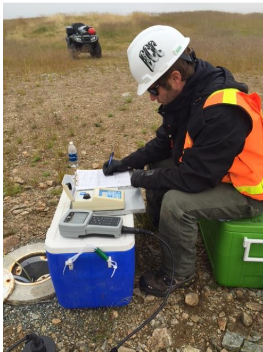
Photo No. 8 – 13 August 2016; 1252 hours. Stability parameter collection at well 14MW06. View facing southeast.
