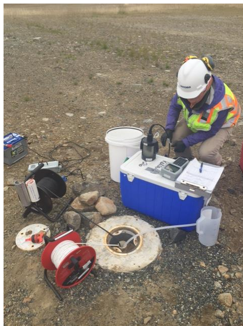
Photo No. 9 – 10 August; 1535 hours. Purging groundwater at monitoring well 14MW01. View facing southeast.
