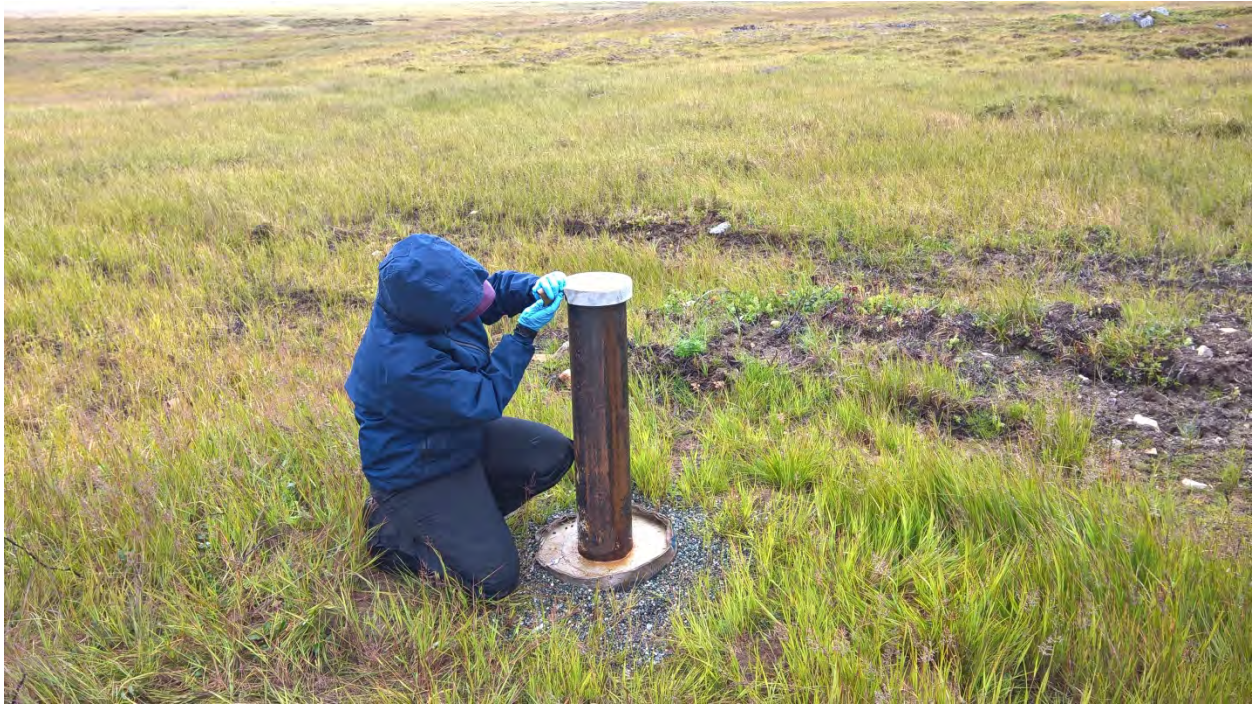
Groundwater sampling – opening stick-up well; View to the north Photographer: E. Barnhill
