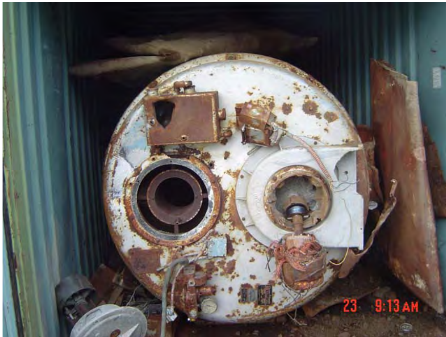
6. Steel boiler with asbestos gasket and asbestos bricks in Conex trailer. BEESC photograph.
