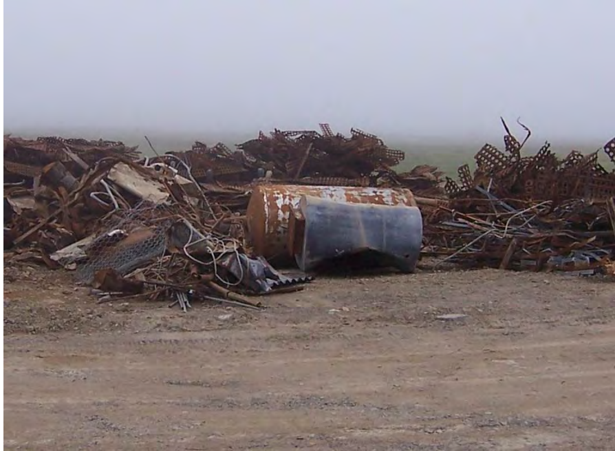
7. Tank with PCB-bearing paint (larger tank, rusted with silver PCB-paint). BEESC photograph.
