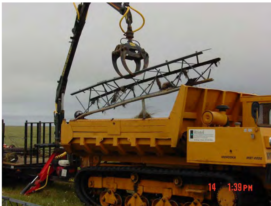
Photograph 26. The log grapple was also used to place various metal towers and poles into Morooka tracked vehicles for transport to the scrap metal staging areas.
