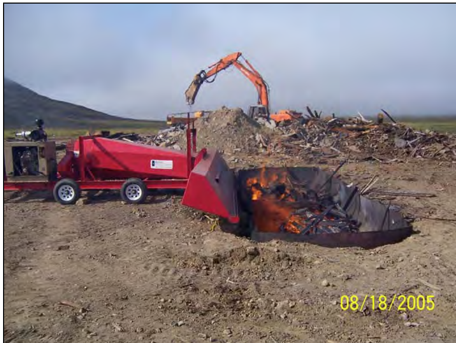
Photograph 32. The burn pit in action. Note that very little, if any, smoke is coming out of the burn pit as a result of the air curtain blower to the left of the pit. Photo facing southwest.
