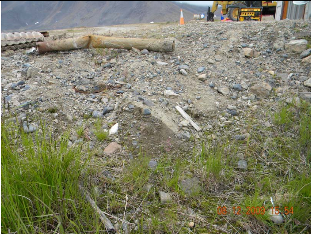
Photograph 18, 8/12/2009, southeast: Injection fluid breakout via sidewall seep.
