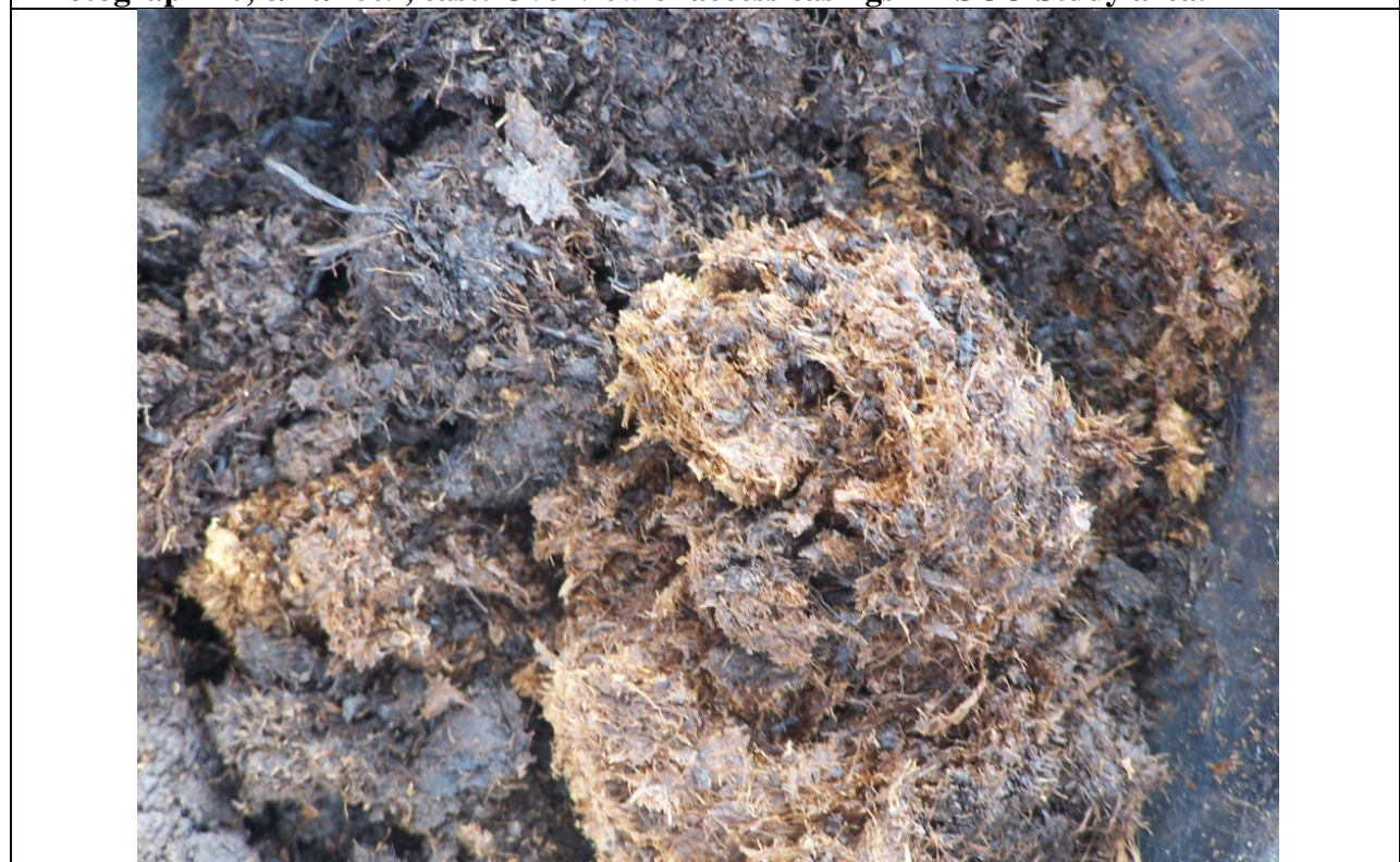
Photograph 21, August, 2009: Post-ISCO HA-3 soils at 5.6 feet below ground surface.
