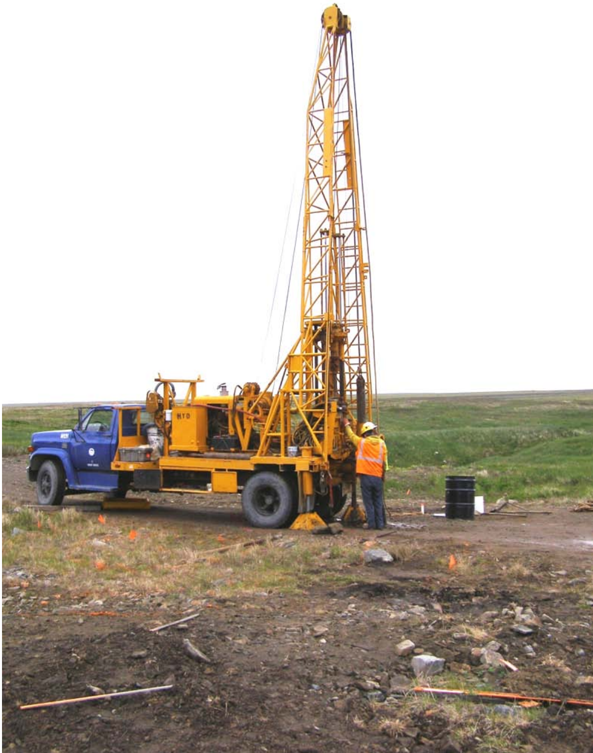
Photograph 7, July, 2009, northwest: Soil boring installation via hollow stem auger.
