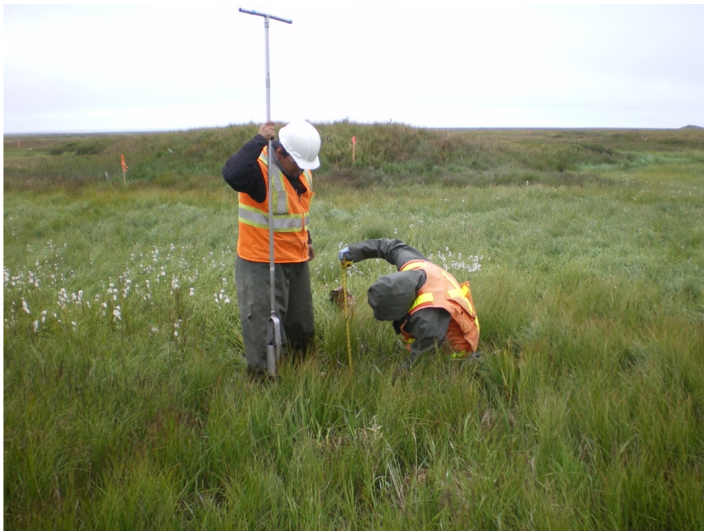
Photograph 4: Measuring the depth interval at a sample location. Direction: Northeast. Date: August 16, 2011.
