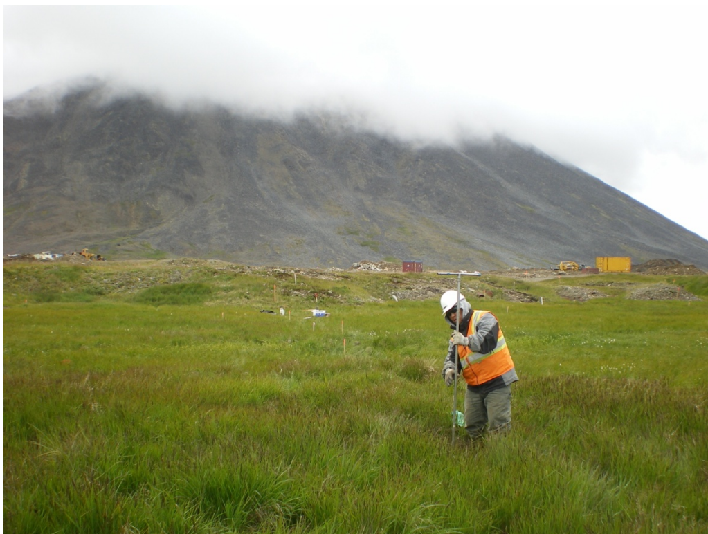
Photograph 3: Local hire Charles Kava obtaining sample material with a hand auger. Direction: South. Date: August 14, 2011.
