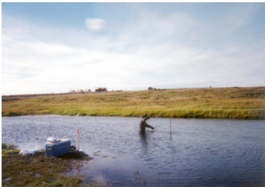
Photograph 14: Sediment samples were collected from depositional areas of the Suqitughneq River Estuary with an Eckman Dredge, looking west-northwest. Tidal influence was not observed in the estuary, which was essentially a fresh water impoundment for the duration of the field activities.
