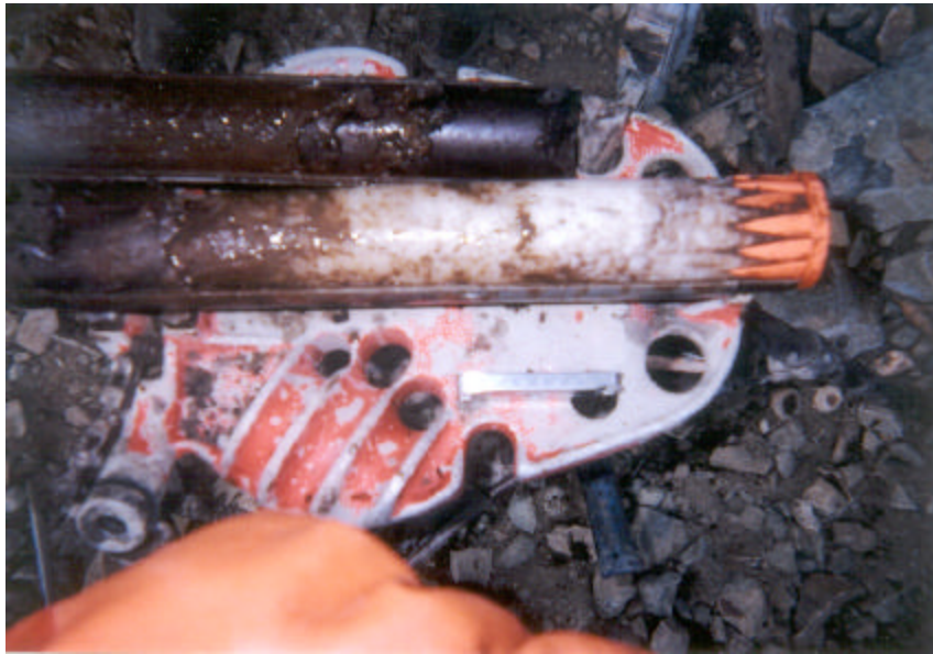
Photograph 5: Ice recovered in split-spoon sampler from 5 feet bgs in Site 3 boring 03B3.
