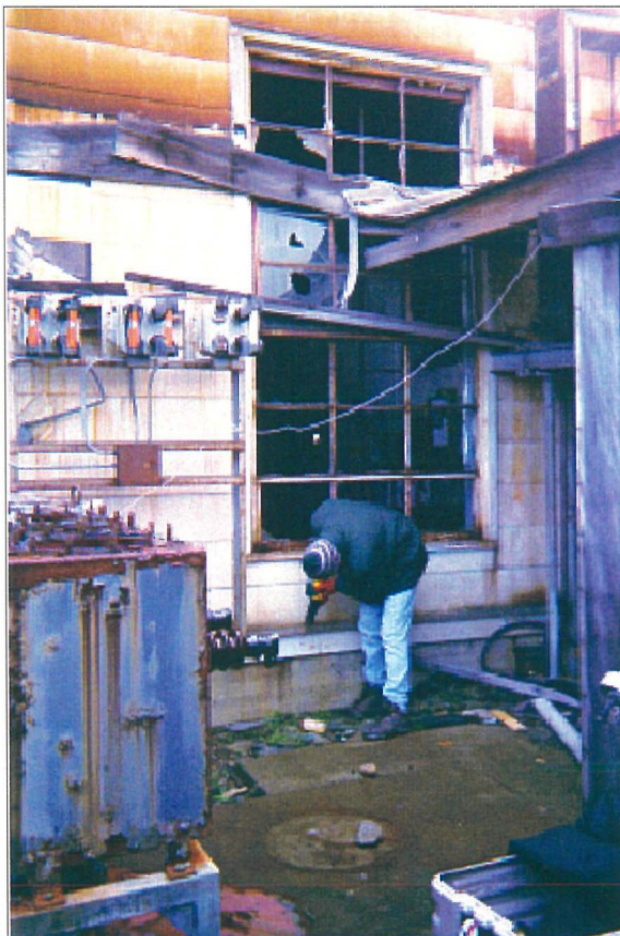
Sampling building materials at Site 13
