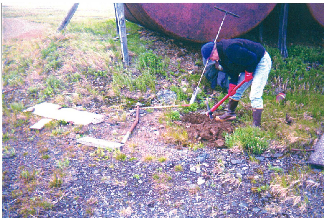
Clearing cobbles before collecting soil sample SS01 at Site 12
