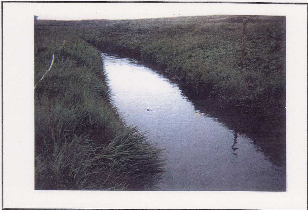
Stream Flow Measurement #8, Near Bridge at Site #2 Note Flotilla - used to time flow avg. of three clockings
